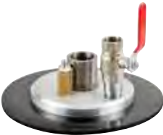
P/N 6048 Follower plate ø 310 mm with NBR seal ring and suction tube adaptor ø 45 mm (for drum with internal ø from 260 to 310 mm)
