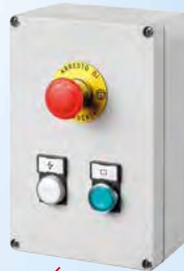
P/N 6047 (to integrate with P/N 6039) Hybrid electric-pneumatic control: features a system discharge timer manually settable, which activates valve P/N 6039
